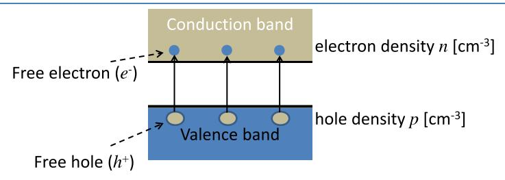
Conduction is due to both electrons and holes in a semiconductor
